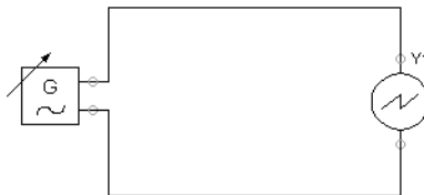
Figure 9/55: Simple circuit with function generator and oscilloscope
